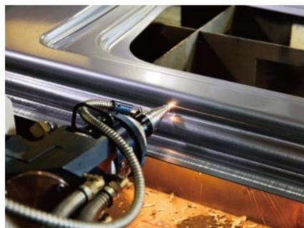
A 3D laser-processing machine machining parts for construction machinery
