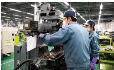
Skills are essentially passed on through OTJ. The photo shows a cemented carbide tool being machined by a worker during OTJ.
