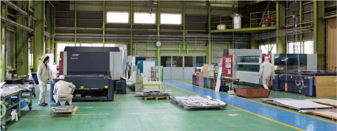
To prevent rust transfer, the ML3015eX-F40 and ML3015eX-60XF—a 6kW CO<sub>2</sub> laser processing machine—are installed in a different building than the other three machines. The ML3015eX-60XF is dedicated to stainless steel cutting.
