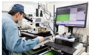
Final inspection prior to shipment. An experienced worker confirms processing accuracy by viewing a microscope image on an expanded display.
