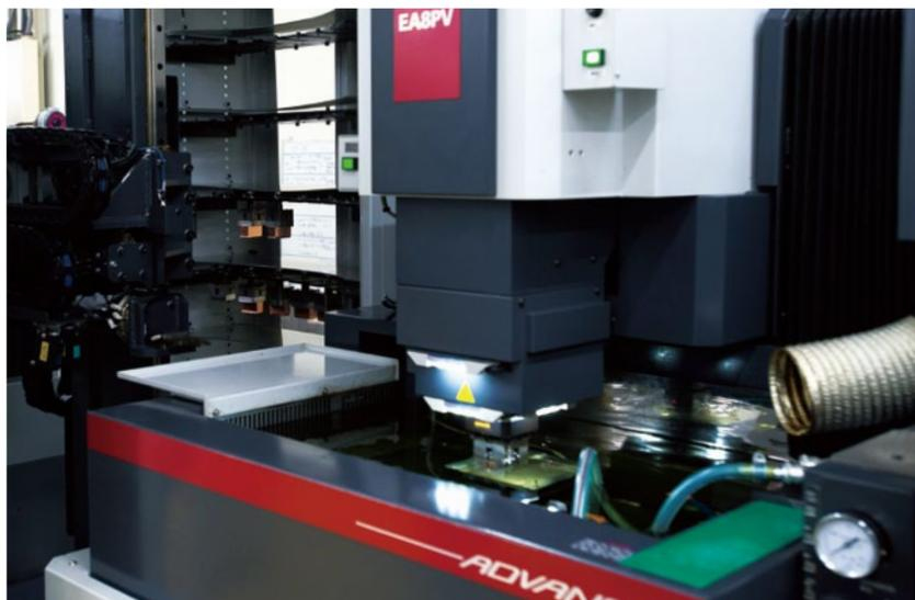
"EASPV ADVANCE" is a die-sinking electrical-discharge machine (EDM) equipped with an automatic electrode changer—called an "ATC"—and workpiece changer. With Mitsubishi Electric's cooperation, the EDM is made to YUWA's specifications.
