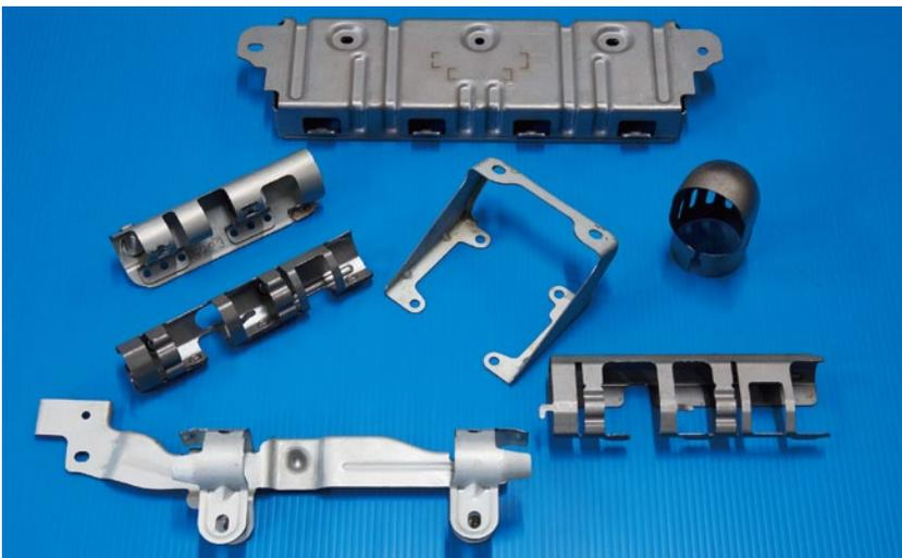
Part prototypes for automotive airbags. These are made by completing the processes of five-stage stamping, bending and curved surface drilling using a 3D laser-processing machine. Tatsumi Seisakusyo is given the freedom to decide the manufacturing methods used.
