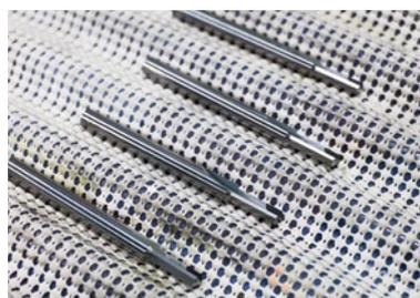
Diamond tools fresh off the manufacturing line. Made by soldering diamond chips onto a cemented carbide tool body.
