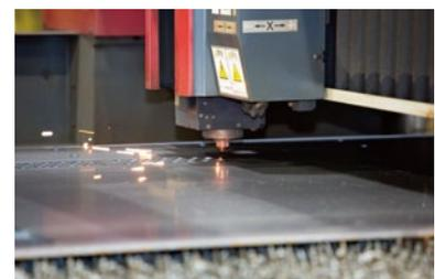
ML6030XL-45CF-R with a power of 4.5kW. Production Manager, Mr. Hirooka, spoke highly of the model saying, “The beams of Mitsubishi Electric’s laser processing machines are good quality.”
