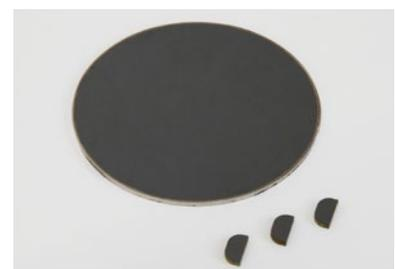
Diamond chips cut from a diamond wafer in a wire-cut electrical-discharge machine.
